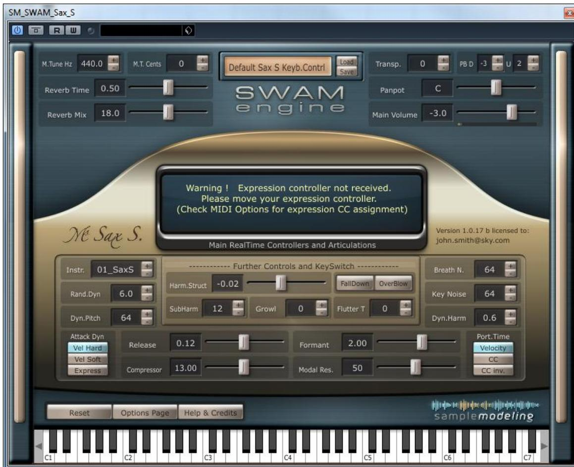
Upon receiving the appropriate CC (from your keyboard or any other midi source, including a wind controller or sequencer) the warning disappears, the current value of the expression CC is continuously displayed in the dynamic envelope window, and the instrument is ready to play.
